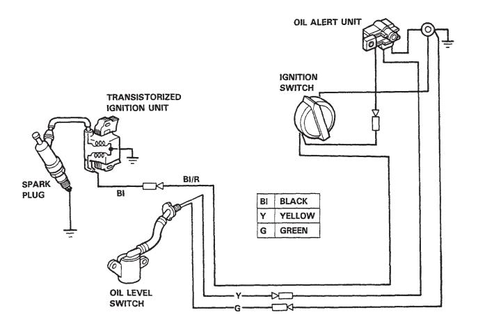
Figure 37. Honda GX270 QWH2 Engine Wiring Diagram
